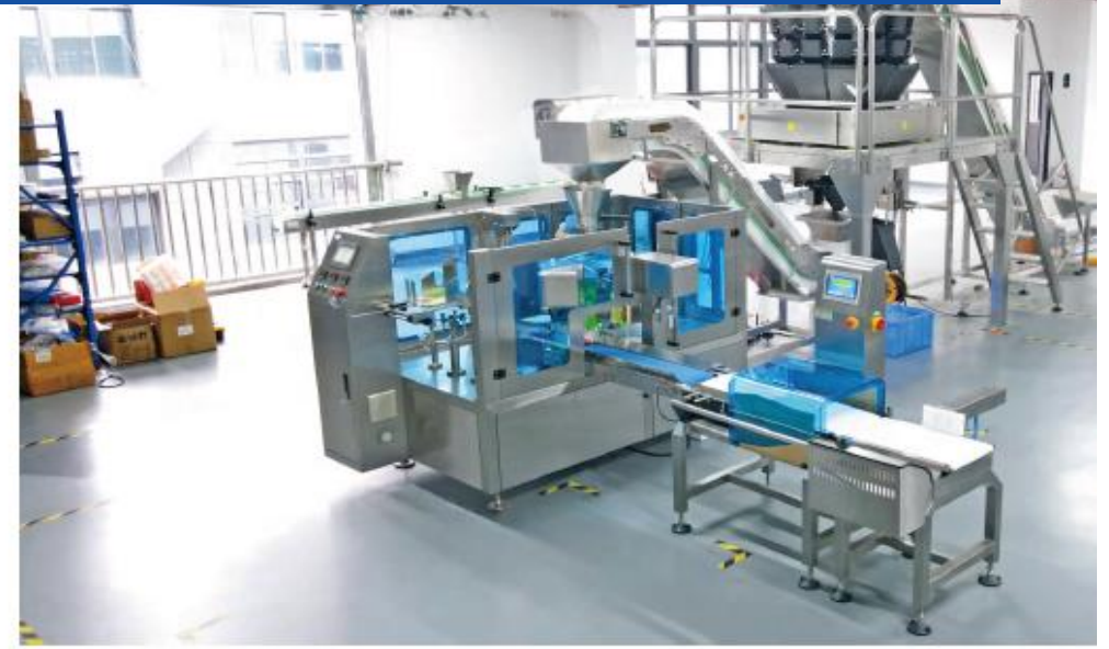
Two level lifting, weighting, packing, inspection
