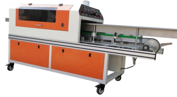
Smart box packer BP030. Wheel rolling glue, high output, easy for changeover
