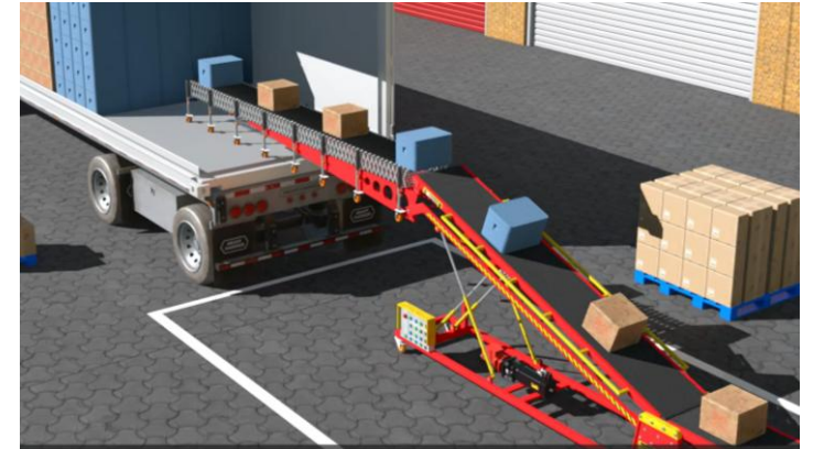
Warehouse ↔ Truck, 2 direction loading/ unloading system
