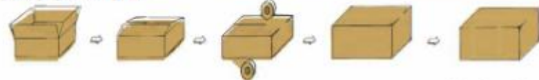
Manually push in → Manually folding → up and down sealing → Sealing finish → Auto Strapping Finish
