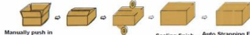
Manually push in → Auto folding → up and down sealing → Sealing finish → Auto Strapping Finish
